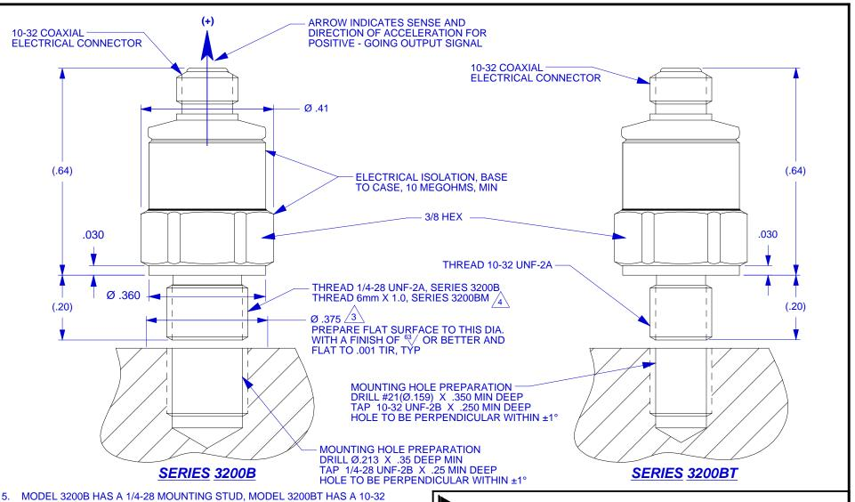
MODEL 3200B HAS A 1/4-28 MOUNTING STUD, MODEL 3200BT HAS A 10-32 STUD AND MODEL 3200BM HAS A 6mmX 1.0 MOUNTING STUD. ALL STUDS ARE .200 LONG.
