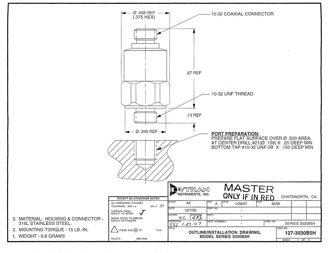
**Model Number** DOC NO PERFORMANCE SPECIFICATION 3030B5H PS3030B5H MINIATURE IEPE ACCELEROMETER REV B, ECN 6906, 07/07/10
