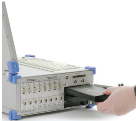
The standard SureHAND has three battery slots already - so adding the 3210-EXP-BATT option provides seven slots total!
