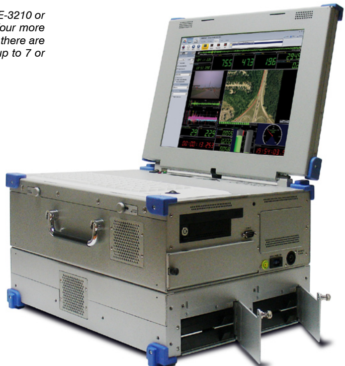
The 3210-EXP-BATT provides four more battery slots
