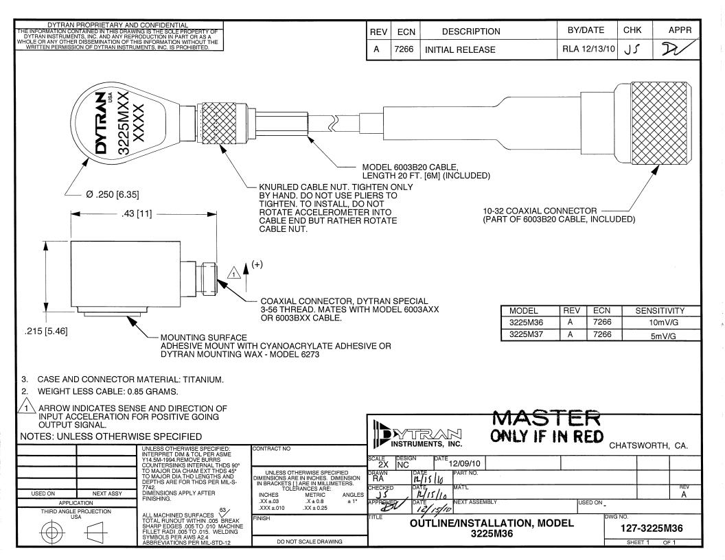
**MODEL NUMBER** DOC NO. PERFORMANCE SPECIFICATION 3225M37 PS3225M37 ACCELEROMETER, IEPE REV A ,ECN 7266, 12/15/10
