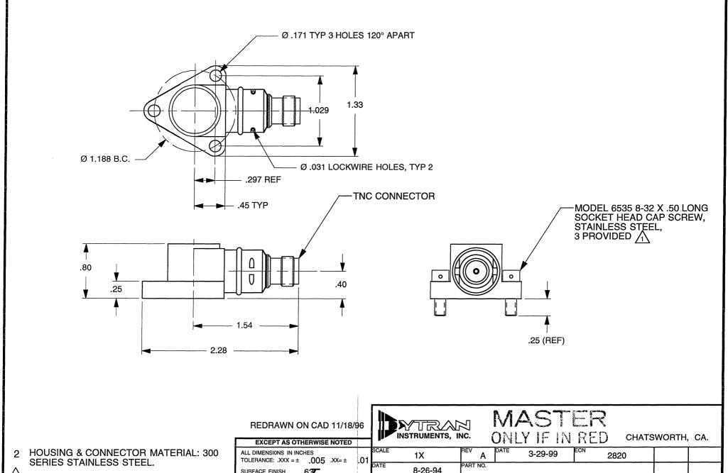
TORQUE MOUNTING SCREWS TO 20 LB-INCHES TORQUE. LOCKWIRE IF DESIRED.
